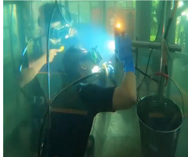
Figure 2 depicts an experiment on underwater welding conducted at a depth of three meters: (A) the underwater welding device is designed to operate at a depth of three meters, and (B) the underwater welding performed via scuba diving.
